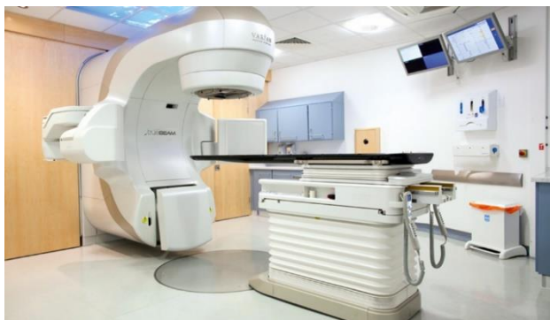
Figure 14. A typical clinical set-up. The linac head (arrowed) rotates around the patient.
