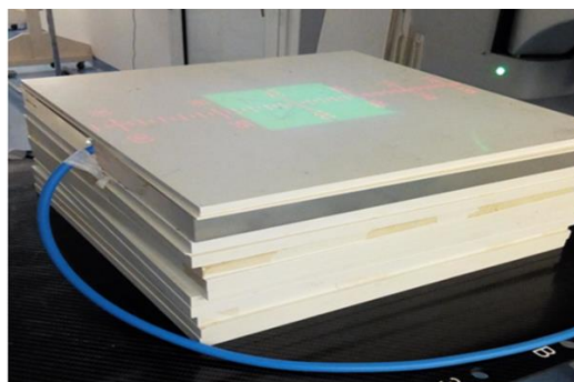
Figure 1 . Set up of the phantom for dose calibration with ionization chamber and Gafchromic.
