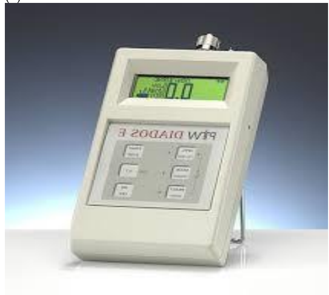
Figure 1. Image of CT ion chamber (A) and electrometer (B) (PTW chamber type 30009, Freiburg, Germany).
