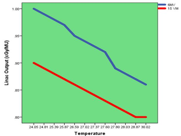
Figure 4. Effect of temperature on photon output of 6 MV and 15 VM over the study period.
