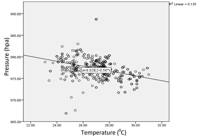
Figure 3. Scattered plot showing correlation between bunker temperature and pressure
