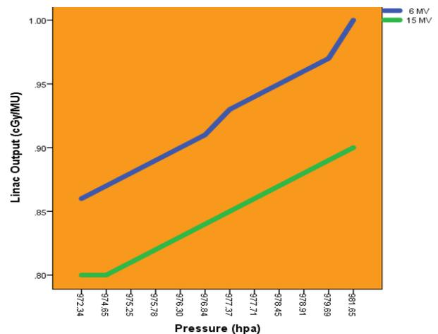
Figure 5. Effect of bunker pressure on photon output of 6 and 15 MV over the study period
