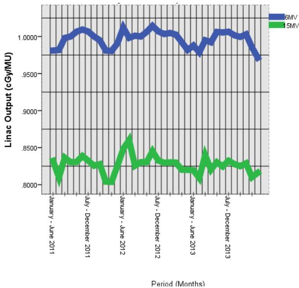
Figure 6. Time history of photon output of 6 and 15 MV from Elekta precise LINAC
