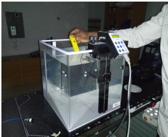
Figure 2. The setup while the pH of the water is being measured.
